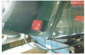
The rear fog lamp is fitted directly onto the rear GRP panel on the off side. There is the option to fit two fog lamps if required, if only fitting one, tape nearside loom and cable tie out of way.
