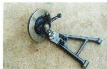
mm bit, you will need to drill through the three holes in ball joint and wishbone together., fitting a bolt after each hole drilled.
