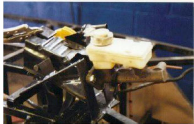
Fig 6a Master cylinder position and is for earlier type sierra master cylinder only fig 6a
