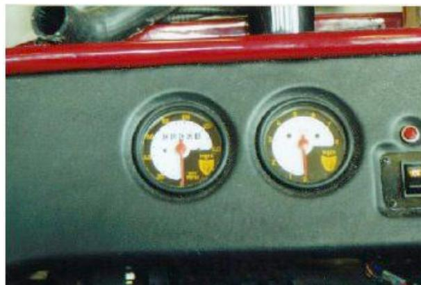
Ensure they can be clearly seen when in driving position, switches should also be reachable. Make sure that the hole measurements are precise, as the front bezel of the fitting must cover the trim cloth to obscure the hole and give a neat appearance.
