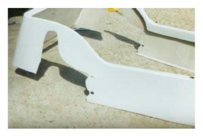
Main Body Tub R6-B6 the standard super six fits the same way With 3.2 holes drilled to attach with alloy rivets .
